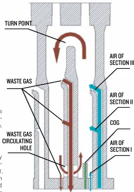
*Schematic diagram of section-wise heating and waste gas circulation*
