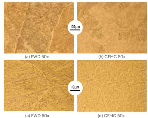
Comparison of crystalline phases of nickel-based superalloy specimens produced by FWD & CFMC
