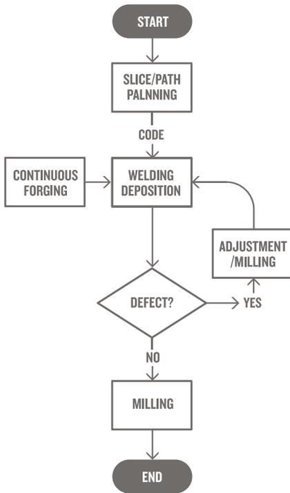
Flow chart of CFMC additive manufacturing
