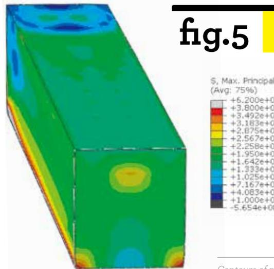
Contours of maximum principle stress in FWD & CFMC specimens
