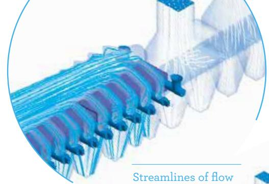
Streamlines of flow in travelling grate
