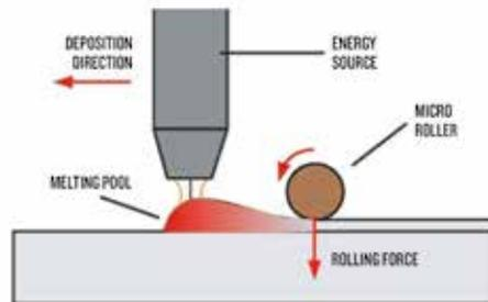
Schematic of casting and forging
