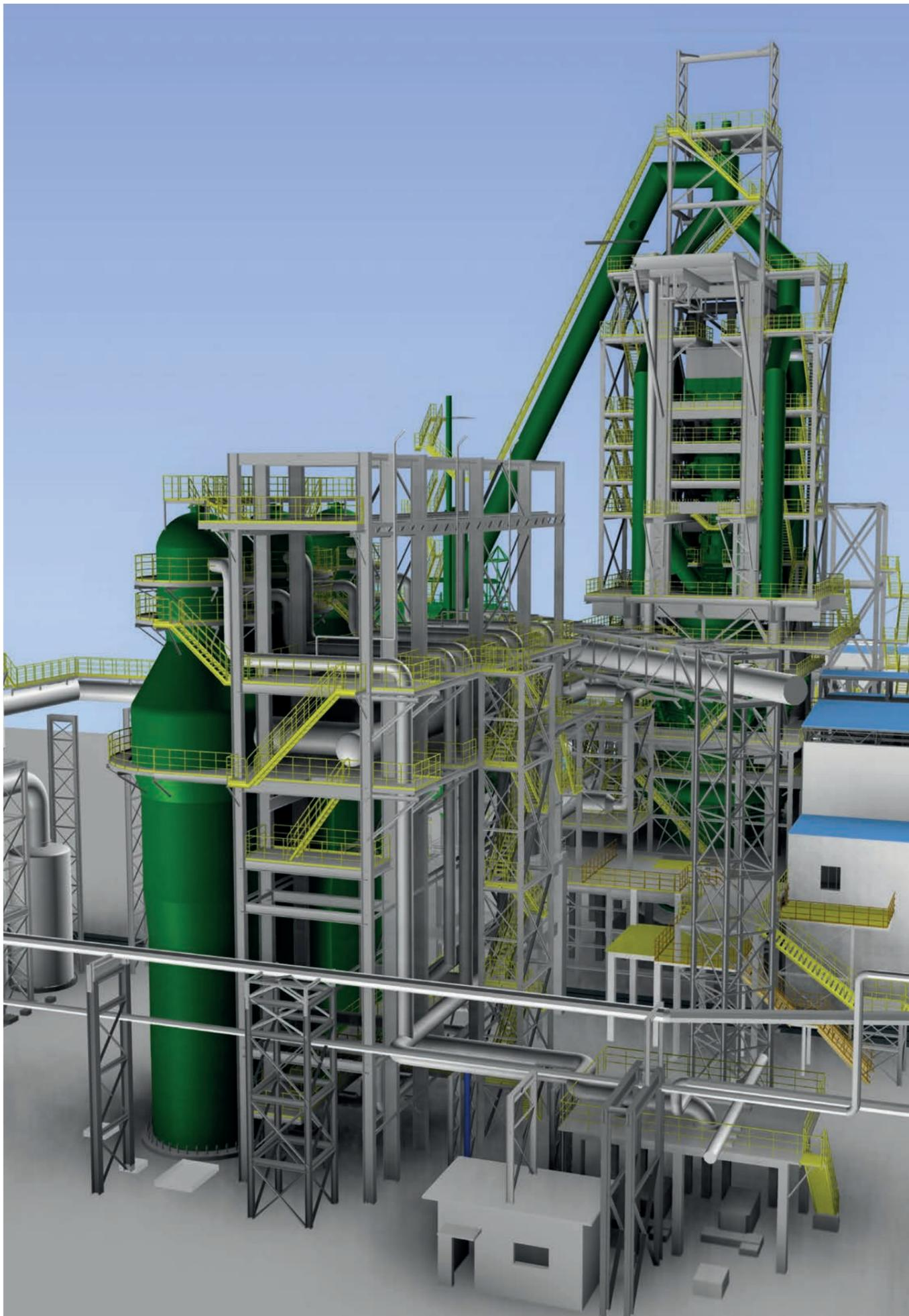
BIM Drawing of Hydrogen-enriched Carbon Recycling Blast Furnace of Bayi Steel, undertaken by Sinosteel E&T
