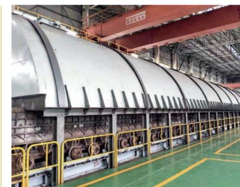
The flue gas circulation systems for three sintering machines have all been put into operation, each with effective ventilation area of 500m<sup>2</sup>
