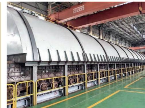
The flue gas circulation systems for three sintering machines have all been put into operation, each with effective ventilation area of 500m<sup>2</sup>
