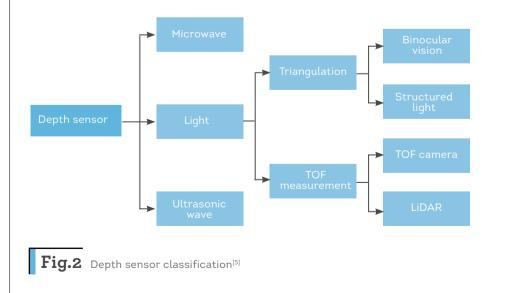
to noise interference, is far inferior to that of a 2D color image; moreover, the TOF camera is high in cost, which to some extent affects its large-scale application. To date, the TOF camera mainly has played a role in fields such as robots, agriculture, healthcare, and industrial automation.
