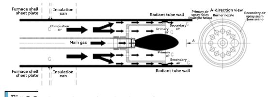
Fig.2.2 Schematic diagram of staged combustion of air
