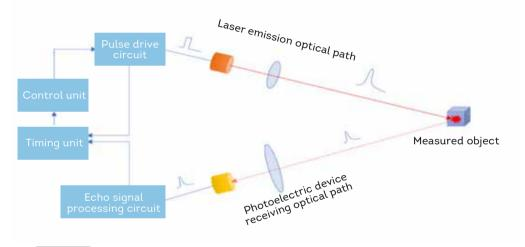
Fig.3 Fundamental diagram of TOF camera
