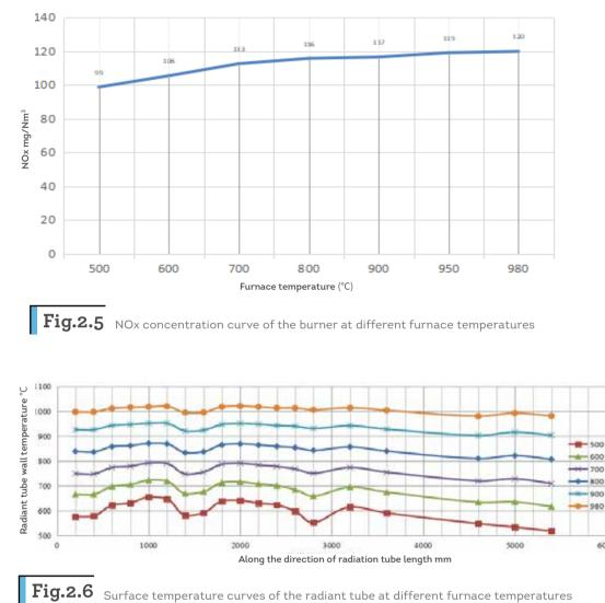
Surface temperature curves of the radiant tube at different furnace temperatures
