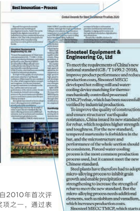
1000-1050°C, provides an alternative solution. Although the rough and medium rolling is conventional, the rolled piece temperature is cooled to the two-phase zone (780-850°C) by pre-water cooling before finishing rolling. Sufficient deformation is applied in the finishing rolling passes, and fine grain rolling is achieved through deformation-induced ferrite transformation and deformation-enhancing transformation.
